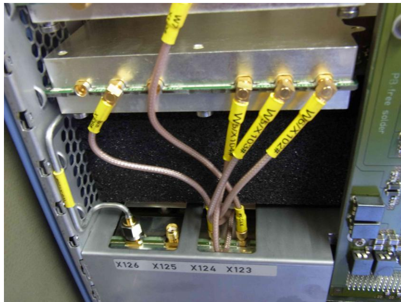
Figure 3-10: Cable routing without option R&S FSW-B71 installed
