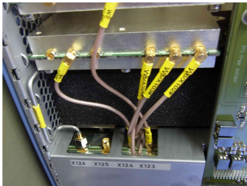
Figure 3-29: Cable routing without option R&S FSW-B71 installed
